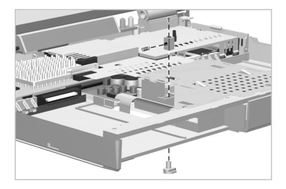
Figure 5-47. Removing the Hard Drive Latch
